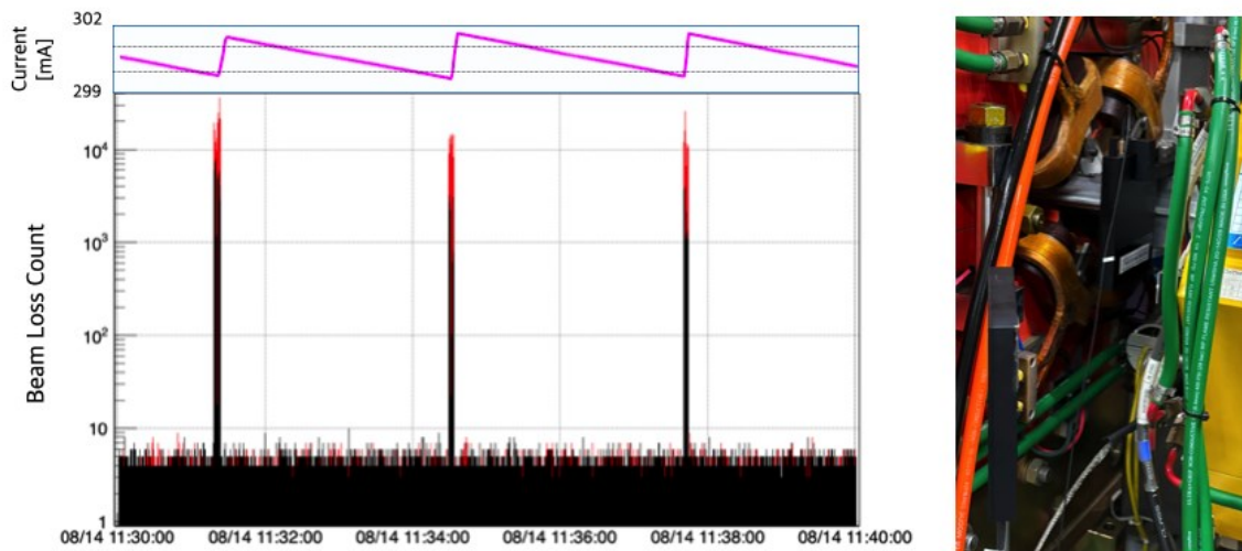
<Figure 2.1.12.39> (Left) The result of Testing at PLS II, (Right) setting up S-BLM on the PLS II beam pipe.
