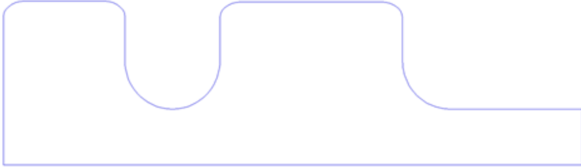
<Figure 2.1.4.23> RF gun cavity designed by SUPERFISH.
