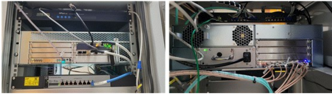
<Figure 2.1.13.22> An example event timing system configured using mTCA.4 infrastructure.
