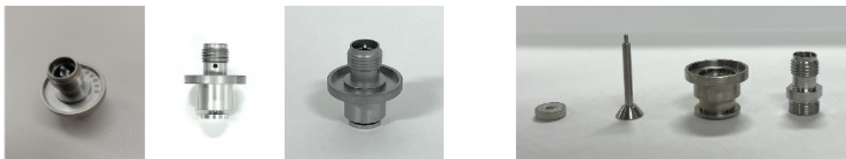
<Figure 2.1.12.22> Prototype sample photo showing two types of pickups for the 4GSR BPM: SiO 2 pickups on the left and Al 2 O 3 pickups on the right.
