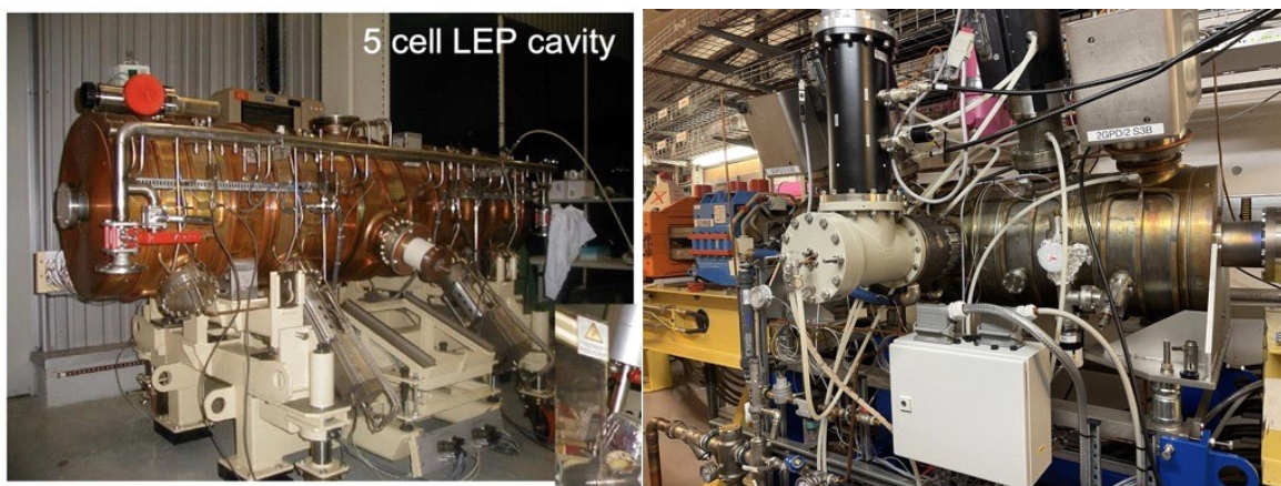
<Figure 2.1.9.34> LEP 5 cell Cavity installed in ESRF-EBS (left), PETRA 5 cell Cavity installed in BESSY-II (right).
